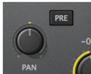
PAN moves the sound left or right, just like your mixer. However the PAN can be automated for auto-panner effects. It can also be placed before or after the stereo width control for a more aggressive auto pan effect. Press the PRE button, and try using an LFO modulation on the PAN position, with the WIDTH set to between 1.5 and 2.0.
