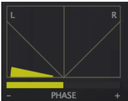
And we can see here the goniometer fully in the out-of-phase area as well. This signal will be trouble. In mono it will vanish entirely as the peaks in the top channel are cancelled out by the troughs in the lower channel.
