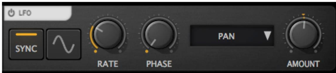
A low-frequency-oscillator (LFO) can be set to control key stereo savage parameters.
