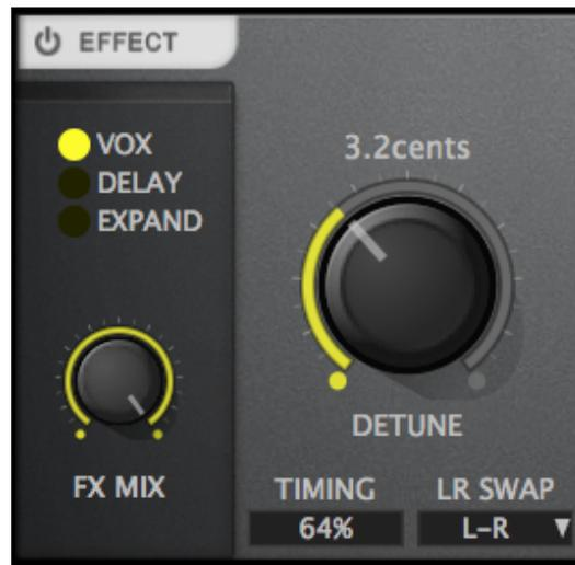
VOX is a special pitch-shift and delay algorithm, popularised by the early pitch-shifting hardware devices from the 1980s and 1990s. It both detunes the left and right channels and adds a tiny bit of variation to the timing.
