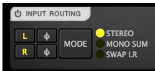
The input routing matrix controls the sound before any processing takes place.
